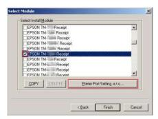
5 The **Printer Port Setting, e.t.c** screen appears. In **Port Type**, Select the port to connect the printer and configure the port setting. Then click the **OK** button.
